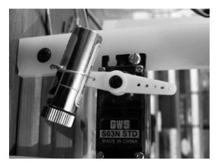
Figure 2-4. Laser diode mounted on servo motor
