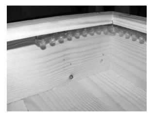
Figure 1-10. The compartment showing LED strip
