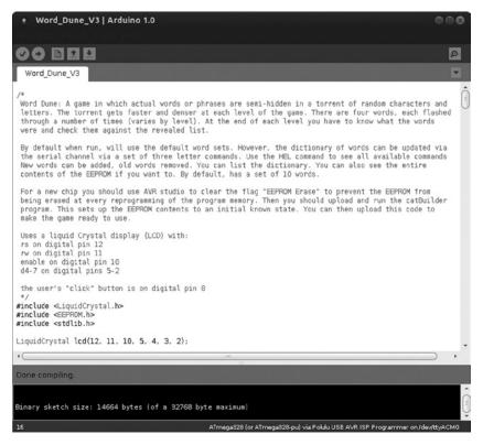
Figure 3-16. WordDune: Word\_Dune\_V3 sketch in Arduino
