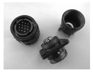
Figure 4-6. Disassembled plug and socket
