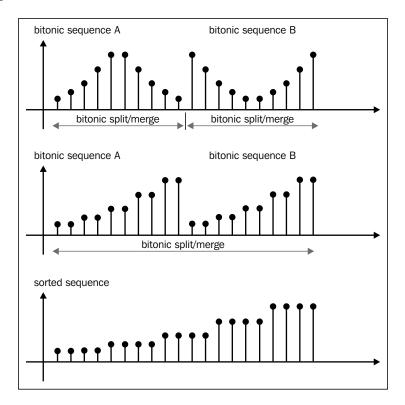
In either case, we will know when to terminate if the split sizes have reached two, because at this point, it's a comparison operation between a and b, where either a is greater than or equal to b or b is greater than or equal to a. And it holds and depending on the sorting order, we will place them into their appropriate position in the output.
