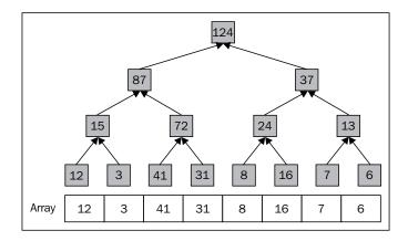
The previous diagram created juxtaposition, and it alters the way the same piece of data you saw, that is, one dimensional flat array containing arbitrary values. Imagine a tree of computations that scans and operates on two values. One way of storing those partial sums is to write the value in place to the array and another way is to use shared memory on the device.
