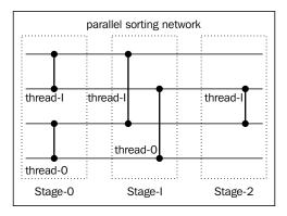
Although it is not the most efficient, the earlier diagram illustrates a possible parallel sorting network for any four keys. In this parallel sorting network, we could potentially launch threads where it will conduct the compare-exchange operations in three stages, and the result is that the input is sorted.
