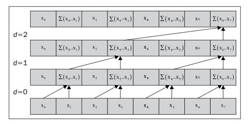
From this diagram, we can observe that partial sums are built up at each level of the tree and one of the efficiencies introduced here is not repeating any addition, that is, no redundancies. Let's demonstrate how this would work for an array of eight elements, and we will also employ the up-sweep algorithm.
