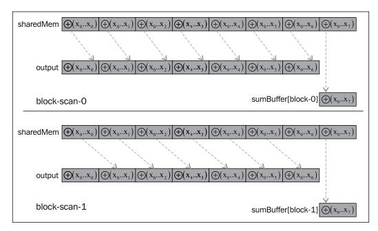
The following diagram illustrates this concept for two parallel block scans (assuming we have a shared memory that holds eight elements) and shows how it's stored into the output:
