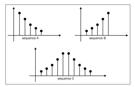
In the situation where we receive an arbitrary sequence, that is, unsorted and not in bitonic order, we have to basically produce a bitonic sequence from this unsorted input and then apply the same trick as before using the bitonic splits until we reach the final sorted state. The following diagram illustrates how a bitonic split or merge (as it's often called) operates on separate sequences and produces the final sorted sequence either in ascending or descending order:
